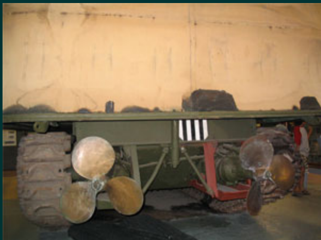
The canvas hull and propellers of a Dual-Drive Valentine.
